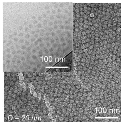
TEM images of 0.1 wt % cationic-modified PGC BCP show spherical aggregates in water. Inset: Cryo-TEM
