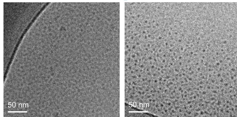
Cryo-TEM image (left) of cationic-modified PGC homopolymers in 100 % H<sub>2</sub>O shows the aggregate formation in H<sub>2</sub>O. Positive staining cryo-TEM (right) is provided to show better contrast. Ammonium Molybdate (16 wt %, pH adjusted) was used the positive staining.
