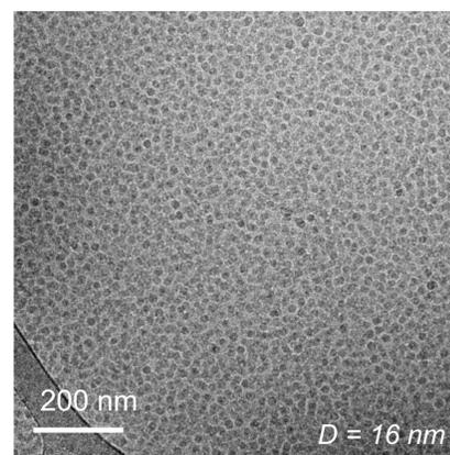
Cryo-TEM image of cationic-modified PGC BCP inverse aggregates in 100 % THF:
