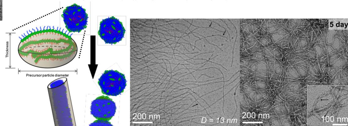
Cryogenic-TEM image (left) shows mature fibril structures with arrows showing twist regions with different density contrast along the fibril. A negatively stained TEM image (right) is provided to show more detailed characteristics such as folds and twists (inset) that are hard to observe from cryo-TEM due to a low contrast from solvent swollen nanostructures.
