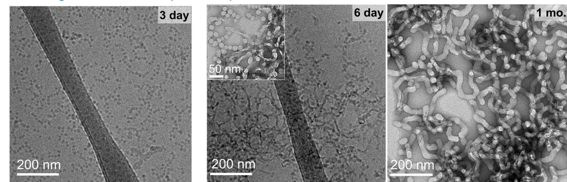
Cryo-TEM image of early assembly stage (3 day aging) is shown on the far left where individual precursors of 10-14 nm diameters are formed. With 6 days of aging, a cryo-TEM image of the intermediate stage shows mixed precursors and loosely formed fibril network structures. 1 month of aging leads to fully mature networks. All regular TEM images are negatively stained for better contrast.
